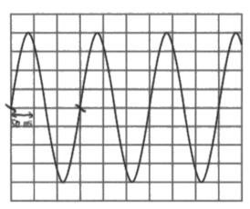
On the horizontal scale of the oscilloscope screen, one division represents 50 ms.
